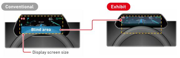
Display area hidden by a steering wheel is shown as a virtual image in the effective area.
