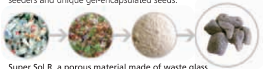
Super Sol R, a porous material made of waste glass
