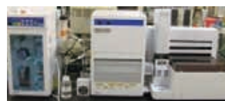
Combustion gas absorber
