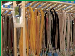
Wiring harnesses are hung in the Store separately for each circuit before they are moved to the next processing step
