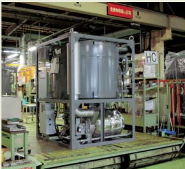
Basic version of the Aroace, to which various functional components are added in a customization process, depending on conditions such as the installation location
