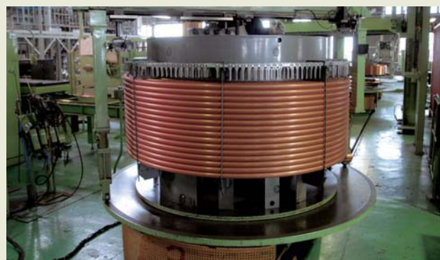
Commercial air conditioners require large-scale production equipment just as cars do. The photo shows the inside of an air conditioner following copper tube installation.
