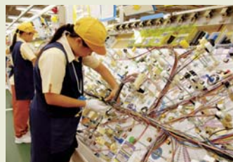
Manually finishing wiring harnesses according to wiring requirements for each vehicle model
