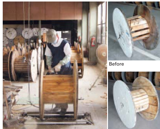
Repairing wooden electric wire spools
