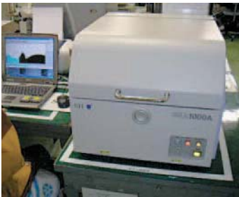
Material tester (energy dispersion type fluorescent X-ray analyzer)
