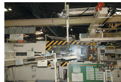
The mold on this 500-ton molding machine is changed in just over 20 seconds
