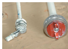
Air curtain-type painting nozzles (Left: Old nozzle; Right: New nozzle)
