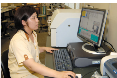
Measuring lead content using an XRF analyzer
