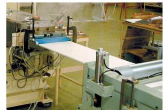
Forming foamed paper board
