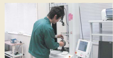
Staff member measuring elongation of an insulator
