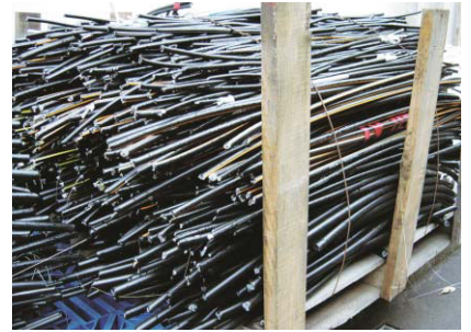
Difficult-to-incinerate aluminum-clad cables at the Hodosawa Factory
