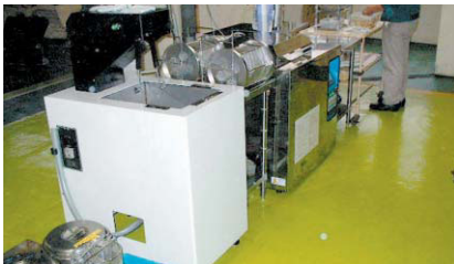
Vibration cleaning system and vacuum dryer
