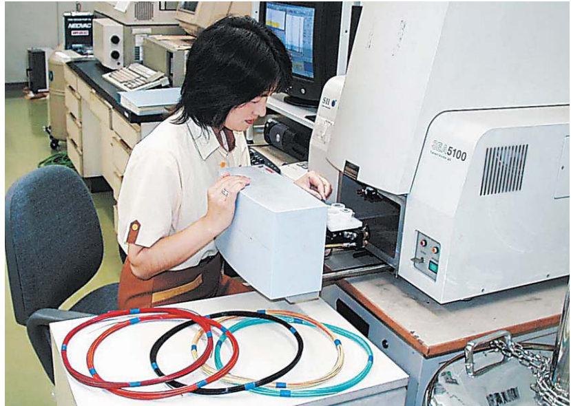
Measurement of lead and cadmium in electrical insulation materials using fluorescent X-ray analysis
