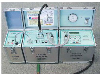
Live wire diagnostic system for 6.6kV XLPE power cables
