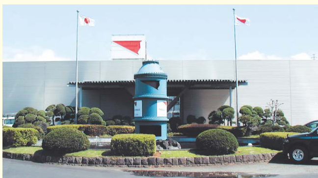
The Thomas furnace (rotary smelter) with greater productivity than the air furnace was first introduced to Japan in 1957
