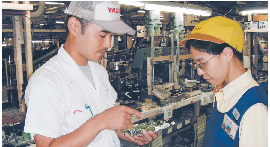
Inspecting the printed circuit board modifications that have been made for a new flat tachograph
