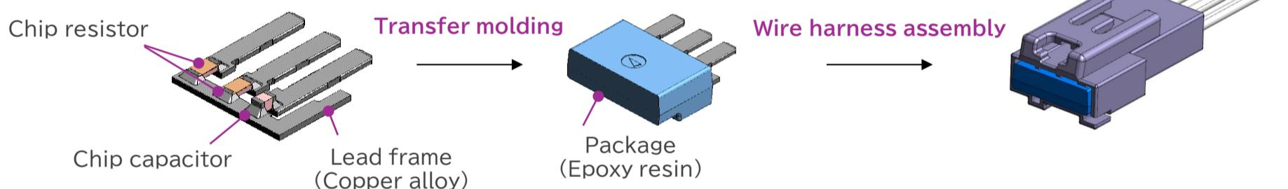
Allows for flexible installation of connectors and electronic components on wire harness circuits
