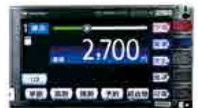
Arofriend 27, a taxi meter compatible with wireless LAN
