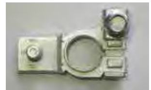
Newly developed product (made by press molding)
