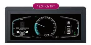
**Basic specification**TFT display (Speed meter, Fuel, Warning lamps etc.)
