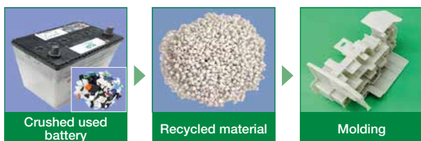
Manufacturing process of connector blocks using recycled PP from end-of-life vehicles
